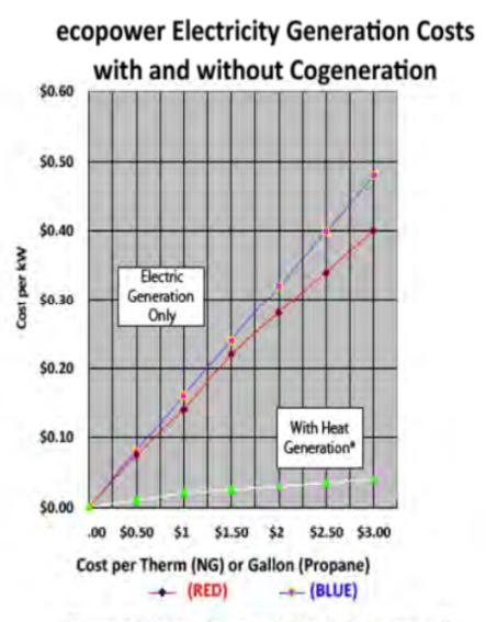
\*Because of the low cost of generation in this mode, both propane and natural gas trend lines are virtually the same.
